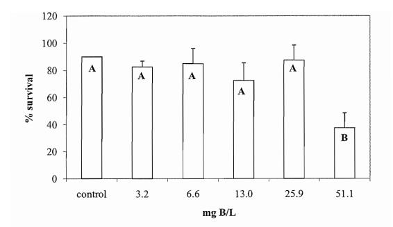
Figure A.3. Mean (error bars = standard deviation) percent survival of *Hyalella azteca* in five boron concentrations and a control (Hard 100b) at the end of a 42-d chronic, static renewal bioassay. Different capital letters indicate means are significantly different from the control (p < 0.05).
