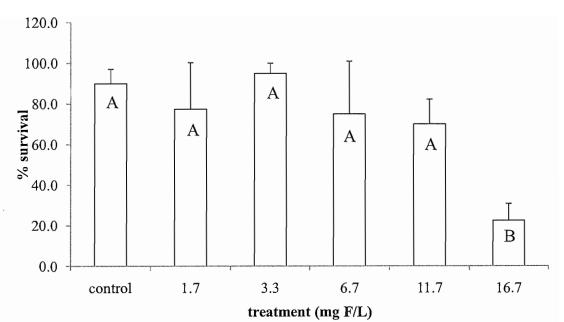
Figure B.1. Mean (error bars = standard deviation) percent survival of *Hyalella azteca* in five fluoride concentrations and a control (Borgmann water) at the end of a 42-d chronic, static renewal bioassay. Different capital letters indicate means are significantly different from the control (p < 0.05).
