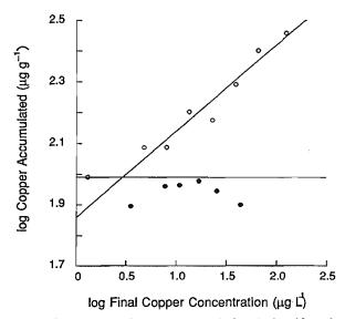
Fig. 5. Comparison of copper accumulation during 10 week chronic (solid symbols) and 1 week (open symbols) exposure to various final copper concentrations. The horizontal line represents the concentration of copper in control amphipods in the 1 week exposure experiment.
