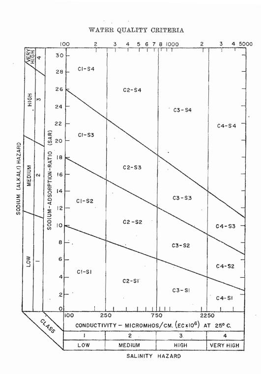
FIGURE 5-1. DIAGRAM FOR THE CLASSIFICATION OF IRRIGATION WATERS (from USDA handbook No. 60)
